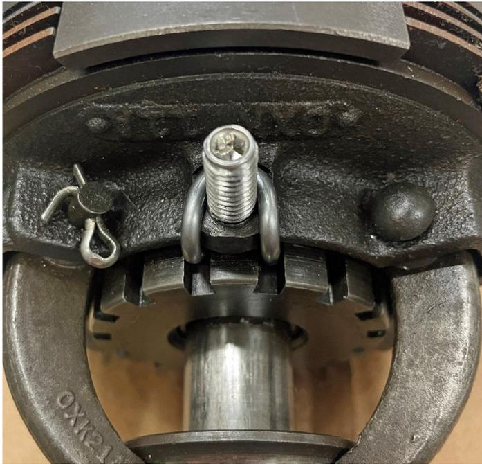
9. Next, land the black flat washer on the stud and push the washer and lock down into the fully seated position using a ½” socket wrench. Once seated, install the silver lock washer.
