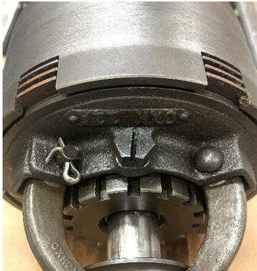
6. Once the original retaining pin is removed, you can readily rotate the Forward adjusting collar CW for more engaging force or CCW for less
