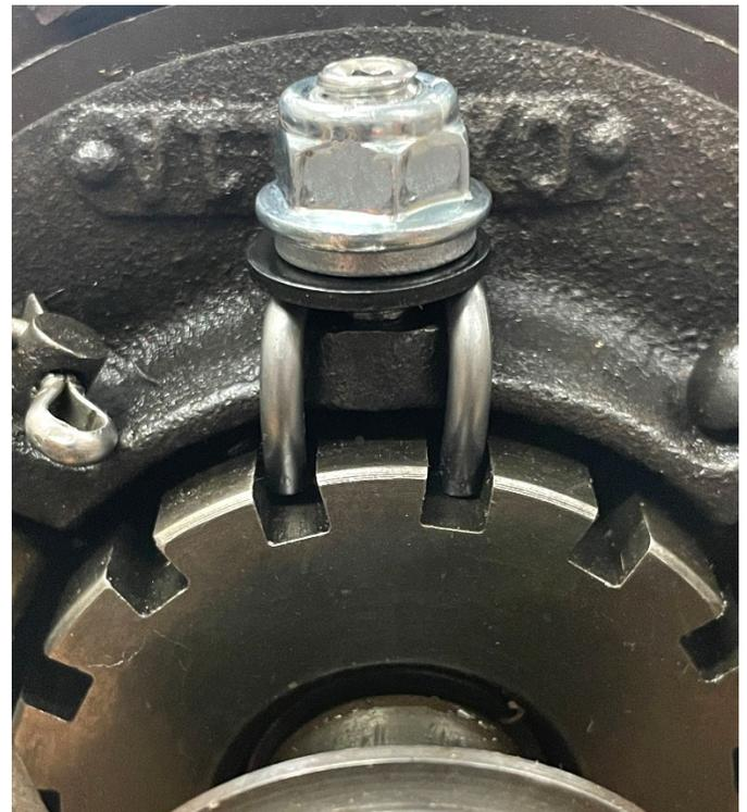
11. Before fully tightening the nut, it is best, if at all possible, to push in against the leg to the right with a screwdriver as you fully tighten the nut as shown to the right. The reason for this is that the lock sometimes wants to rotate as a result of the torque being applied by the washers under the nut. Fully tighten the nut. If a screwdriver cannot be utilized, the installation will still be acceptable. The lock may just rotate slightly
