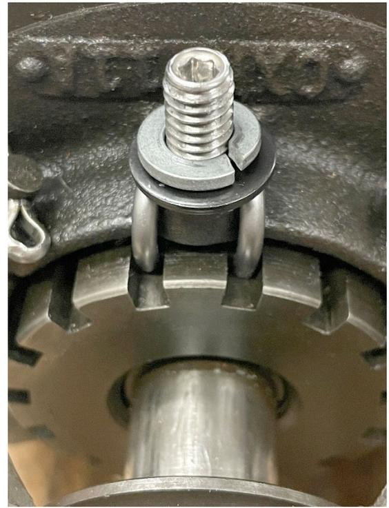
10. Next, thread the Self-Locking nut onto the stud. You will be able to screw it down with your fingers until the threads of the stud engage the nylon element in the nut. At that point, a ratchet with a ½” socket is the best way to screw the nut down farther.
